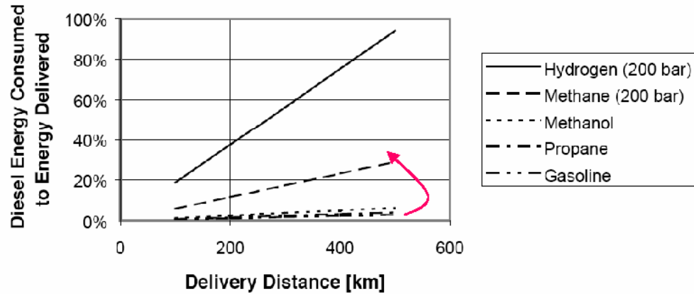
Relative Energy Consumption for Road Delivery of Energy
