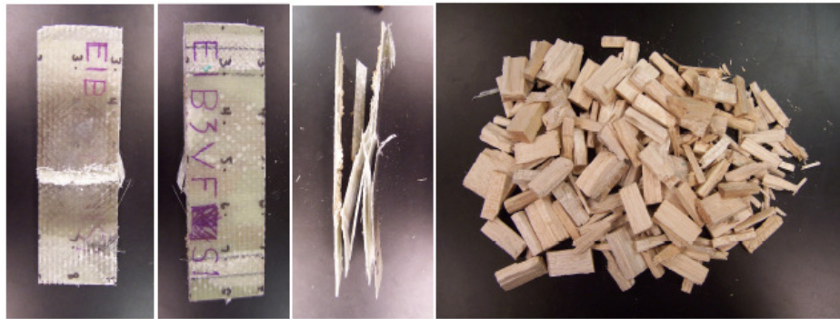
(a) Shock face, (b) back face, and (c) left side view of E-glass/Balsa sandwich composite; and (d) the splintered balsa core pieces after shock testing at 1200 psi (1340 m/s).
