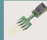
Embedded moisture sensor SH75
